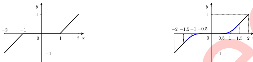
Figure 2 Ideal dead zone and pseudo-dead-zone D_{1,2}(x) , left and right, respectively. For D_{1,2}(x) , it is associated with Q_{\frac{1}{2},2}(x) = -\frac{1}{2}x^4 + \frac{3}{4}x^2 + \frac{1}{2}x - \frac{3}{32} ; the blue curve segments in the first and third quadrants are generated by functions -\frac{1}{2}x^4 + 2x^3 - \frac{9}{4}x^2 + x - \frac{5}{32} and \frac{1}{2}x^4 + 2x^3 + \frac{9}{4}x^2 + x + \frac{5}{32} , respectively.
